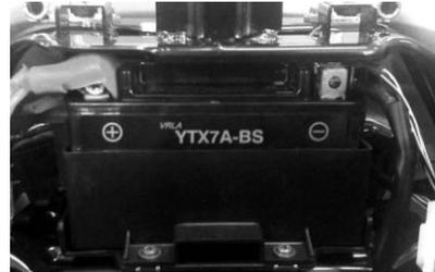
4. Two black grounding cables connected to the battery's negative terminal should be securely fixed to the ground stud, or the engine cannot be started.
