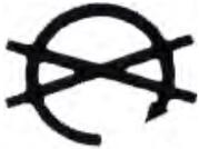
All the power is cut off. The key can be pulled out from this position.
