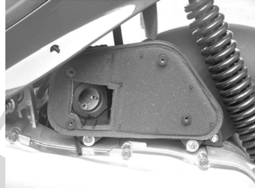
If the air filter element is clogged, it will reduce engine performance and cause abnormal fuel consumption.
