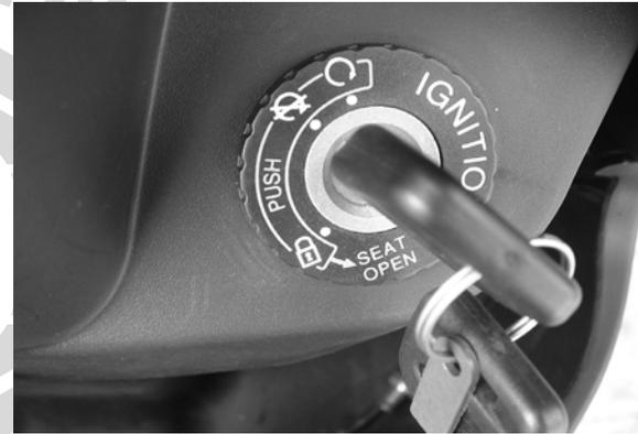
All the power is cut off, and the handlebar is locked in this position.
